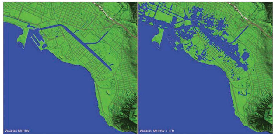
Figure 3-17 Waikiki District: Areas shaded in blue on the left lie at or below 0.3 m above the current high-tide line; areas shaded in blue on the right lie at or below 0.9 m above the current high-tide line. The thin white line is the current shoreline. (Courtesy of University of Hawai'i Coastal Geology Group.)
